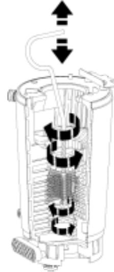
Clean around sealing surface on sump and replace access cover (Q). Using a suitable container to collect water from syphon connection at the base of the boiler flush heat exchanger with water.
