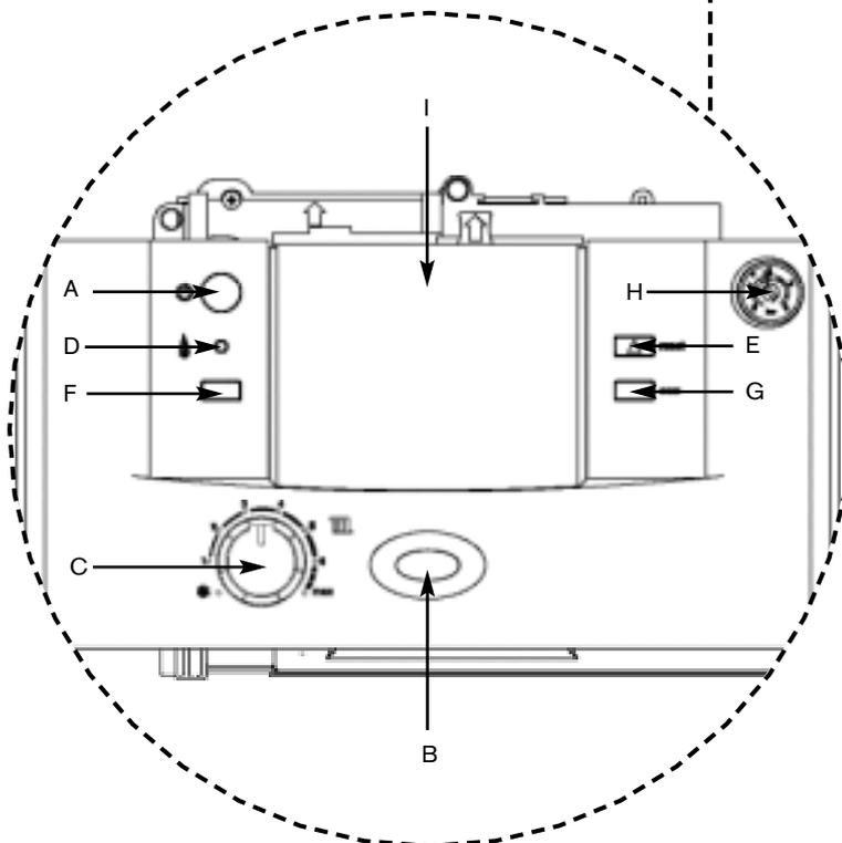
**CAUTION: DO NOT PRESS POWER INDICATOR (B) TO RESET BOILER.**
