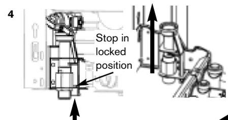
Do not lift by the air gas manifold.
