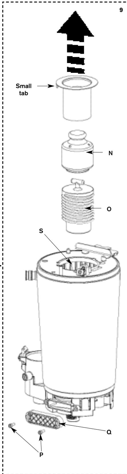
**IMPORTANT: IF THE JOINT BETWEEN THE AIR/GAS MANIFOLD AND THE HEAT EXCHANGER IS DISTURBED THE SEALING GASKET MUST BE REPLACED.**
