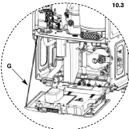
The following components require the air / gas manifold and fan assembly to be removed:
