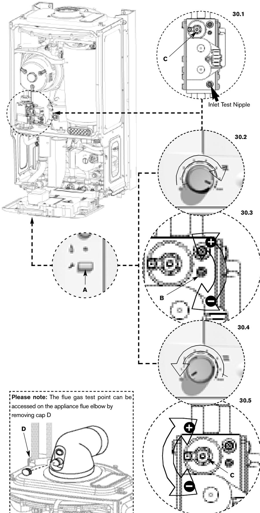
**Please note:** The flue gas test point can be accessed on the appliance flue elbow by removing cap D
