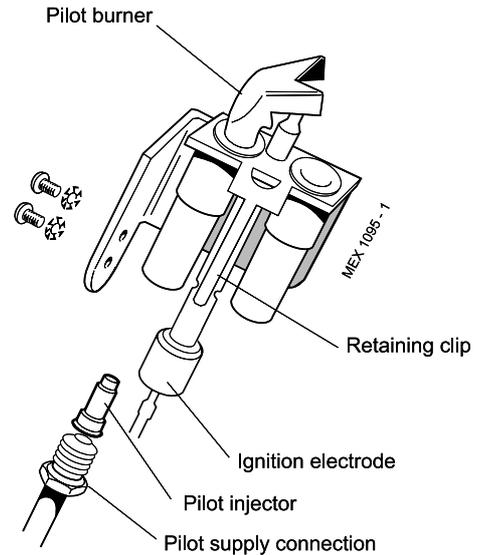
4. Push in the new electrode until the retaining clip locates in the groove and re-assemble in reverse order.
