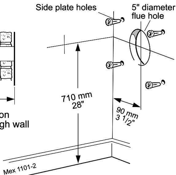
**Note.** If the terminal is to be sited within 25-40mm of a corner or vertical pipe (refer to Table 3) then the hole **MUST** be accurately cut and the rubber weather seal trimmed around the groove provided. The terminal wall plate need not be fitted.
