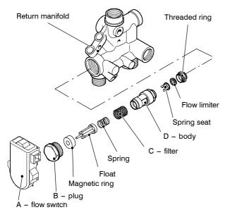
Attention: the magnetic ring has a magnetic polarity and must be correctly coupled with the spindle of the float.
