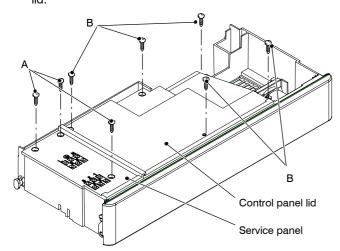
5 Remove all the wiring connected to the main control p.c.b. To disconnect the connectors indicated, delicately flex the hook present on one side of each socket.
