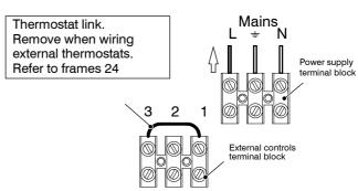
Note: Ensure that the lengths of the current conductors are shorter than the earth conductor so that if the cable slips in its anchorage the current carrying conductors become taut before the earth conductor.
