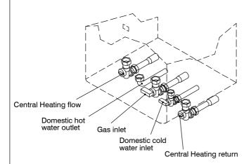
Connect to the tail pipes by proprietory fittings.
