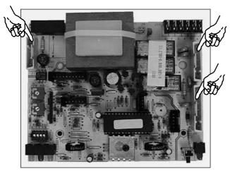
6 Remove the spindles of the CH and DHW temperature adjustment knobs by delicately pulling them with pliers in the direction shown by the arrow.
