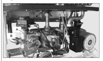
5 Re – assemble in reverse order. Refer to the following illustration for the correct wiring connectors on the switch
