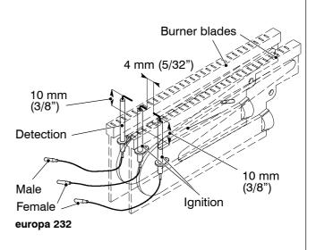
9 Check that the spark and detection electrodes leads are in good condition and renew as necessary.
