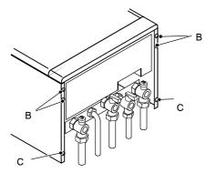
4 Remove the side panels or move the lower part of the side panels and pull the control panel.
